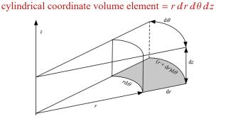
You typically want to match your coordinate system to the geometry of the problem. Hence, you tend to you spherical coordinates when working with spheres and cylindrical coordinates in problems with rotational symmetry about one axis, such as in this next problem.
